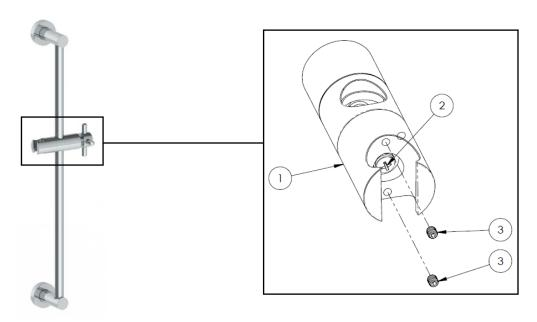
To decrease the stiffness of the positioning bar slider (1), turn each set screw (3) counter clockwise in ¼ turn increments until the desired stiffness is achieved.
